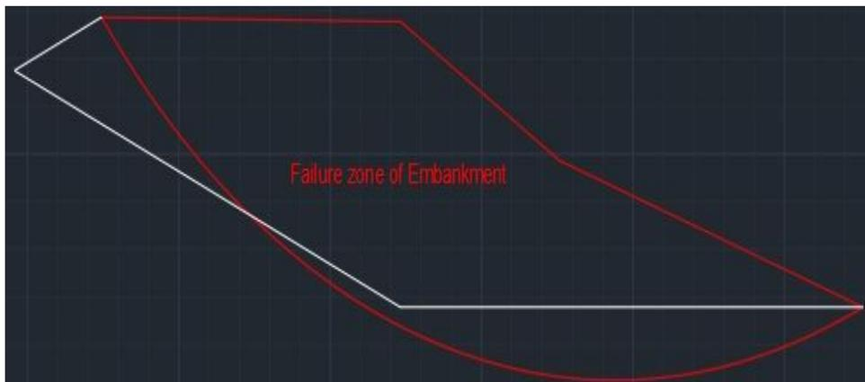
Figure 11: Failure zone of embankment obtained from AutoCAD
